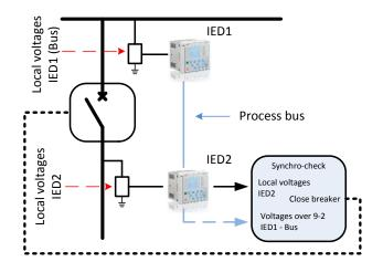
Figure 4. Synchro-check function configuration
