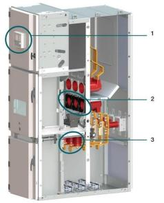
Figure 6. Cross section of a Digital medium voltage switchgear panel (1 - protection relay with IEC 61850, 2 - current sensor, 3 - voltage sensor)
