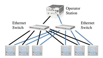
Figure 2. Redundant PRP network.
