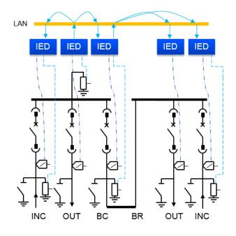
Figure 1. Combined station and process bus
