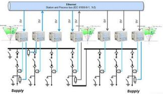
Figure 7. Synchro-check application in switchgear with single busbar arrangement in two bus section arrangement
