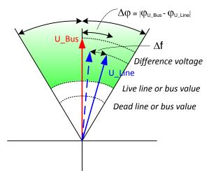
Figure 2. Conditions to be fulfilled when detecting synchronism between systems (phasor diagram)
