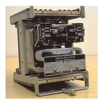
Figure 2 An electromechanical relay
