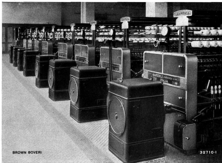
Fig. 22. — Drive of cotton twisting frames by three-phase commutator motors, type PD 126.
