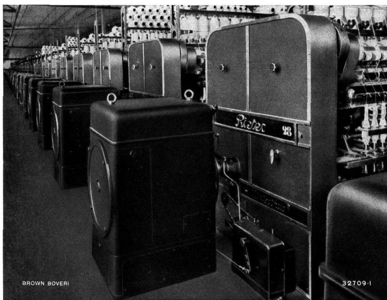
Fig. 20. — Drive of cotton ring spinning frames by three-phase commutator motors type PD 126.
