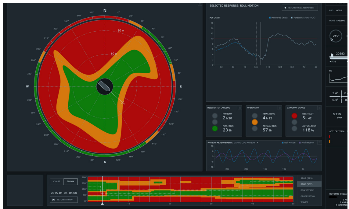
Figure 1: Display indicating the response envelope as a function of vessel heading. Using this display, the operator can easily find the optimum heading, i.e. the heading where the motion response at the crane tip is at its minimum (for example).
