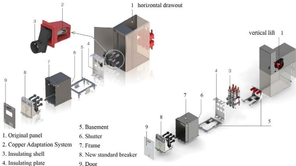
Fig. 4 Innovative retrofill for horizontal drawout and vertical lift original switchgear design components
