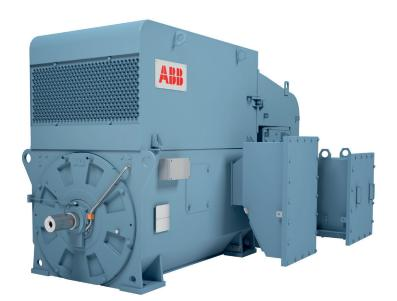
Slip-ring motors are an ideal solution for applications which require high starting torque and low starting current. They are especially suitable for heavy load inertia applications like mill drives or situations where network conditions are weak.
