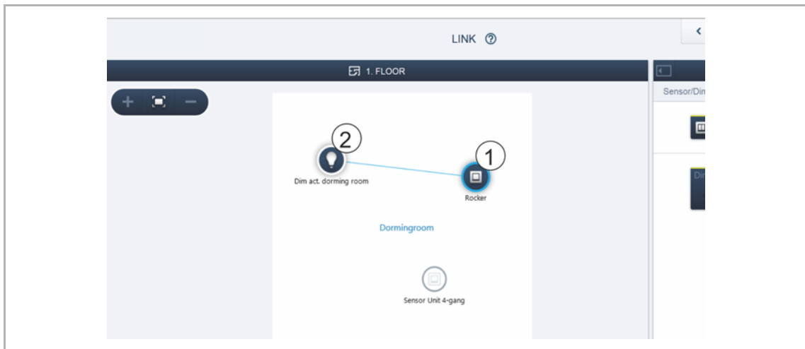
Fig. 22: Linking actuator and sensor
