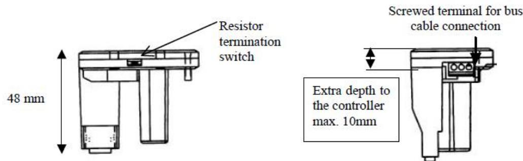
**CAUTION:** Be careful that the RS485 MODBUS ADAPTER is the one with a GREEN text colour (3.3V power supply). The one with a WHITE text colour is reserved for the old model (5V power supply).
