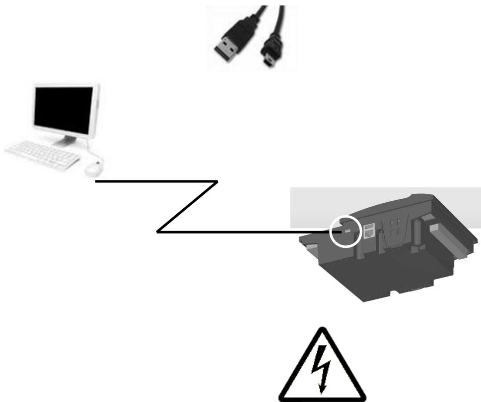
**Caution:** The USB connection to the RVT is not isolated. It is mandatory to connect the protective EARTH connection when using the USB.
