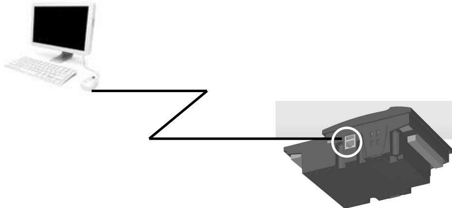
The RVT can be connected directly to a LAN or through Internet
