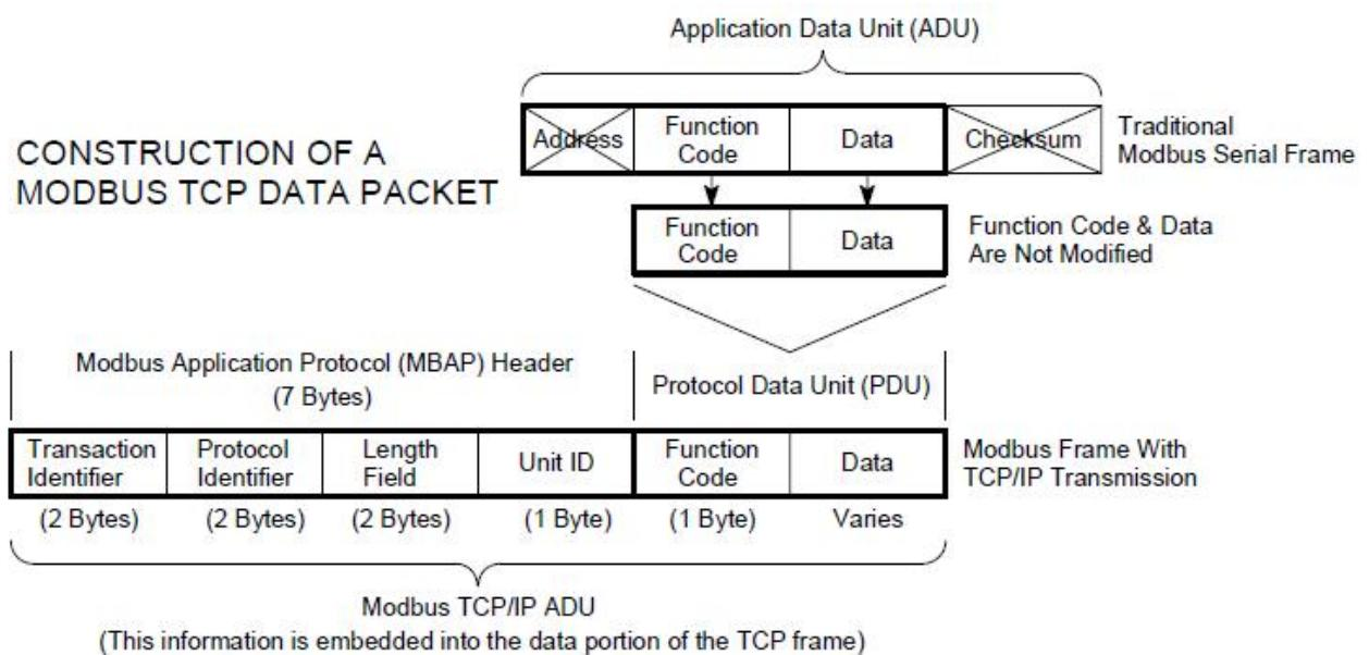
The complete Modbus TCP/IP Application Data Unit is embedded into the data field of a standard TCP frame and sent via TCP to well-known system port 502, which is specifically reserved for Modbus applications. Modbus TCP/IP clients and servers listen and receive Modbus data via port 502.
