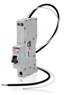
With its breaking capacity of 10kA in only one module width and 115mm height, DSE201 M series is the perfect solution for a complete protection in commercial and industrial applications, where space optimization is particularly required. The unique earth fault indicator window identifies any earth fault trip, making easier the troubleshooting on the network and reducing the downtime for maintenance.
