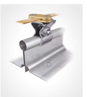
The Furse circular standing seam holdfast range offers air rod bases, conductor clips and square clamps suitable for securing the most common conductor types, 25 x 3 mm tape and 8 mm diameter solid circular, to circular standing seam cladding systems.
