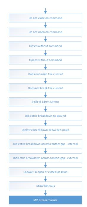
Fig. 2 MV breaker as series of failure modes.
