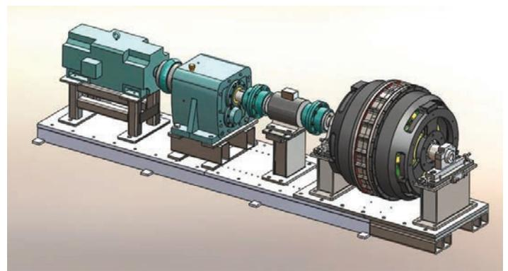
Figure 2: Electromagnetic simulation of the full generator. | Figure 3: exploded view of generator. | Figure 4: Test bench with drive machine (left) and generator (right). Gear box and torque transducer are also shown
