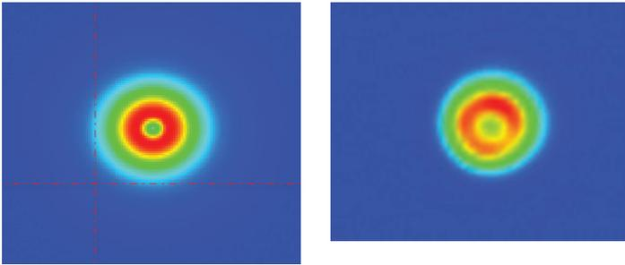
Figure 5: Virtual Applicator Stationary Spinning Atomizer Profile. Top View in 2D. | Figure 7: Simulated Stationary Spinning Atomizer Profile. 3D View.
