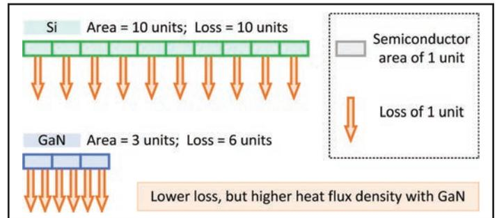
Figure 4: Illustration of the thermal management challenge with GaN
