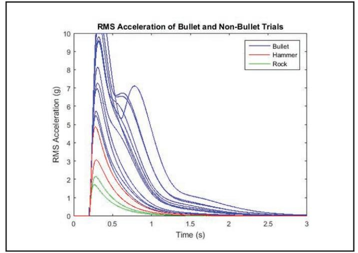
Figure 1: Impact on a test object during a UL-9 trial | Figure 2: RMS acceleration for bullet trials
