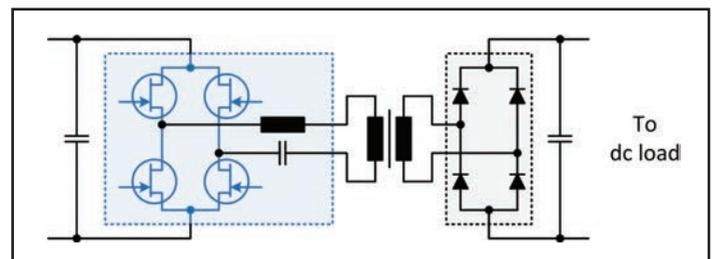
Figure 3: LLC resonant converter using GaN
