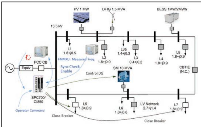
Figure 1: Integrated microgrid protection and control functions for resynchronization.
