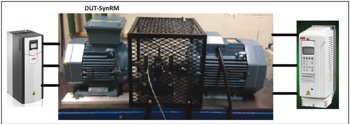
Figure 1: Experimental Setup: SynRM driven by an ABB low voltage (LV) AC drive coupled to an IM
