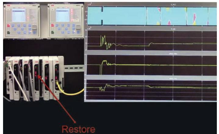
Figure 2: HIL Simulation results – unplanned islanding and resynchronization.
