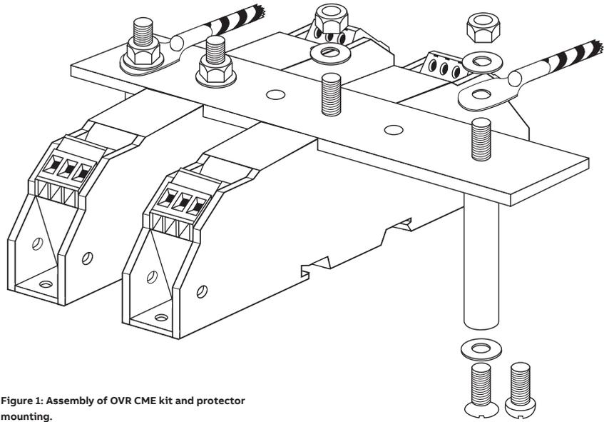
**Figure 1: Assembly of OVR CME kit and protector mounting.**
