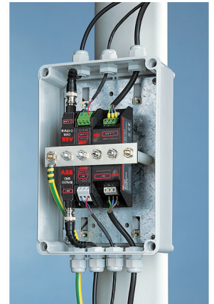
Figure 11: For outdoor installations the OVR SPD should be bonded to the power earth. The CCTV video line and the control line SPDs are connected to the mains power line protector, and hence the power earth, via the CME 4 earth bar. This, in turn, is cross-bonded to the mast or pole.
