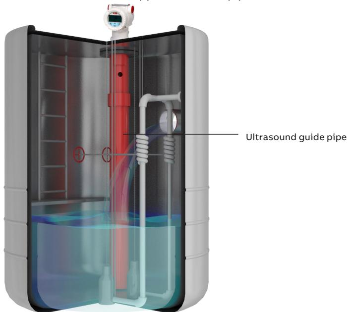
Figure 18 Ultrasound guide pipe installation
