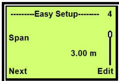
7 Press **Next**. to confirm the Span configuration.
