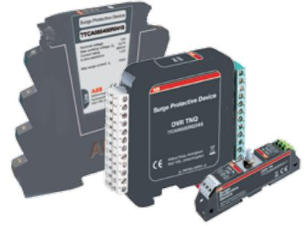
Combined Category D, C, B tested protector (to BS EN 61643) specifically designed for telecommunications applications in accordance with Telcordia and ANSI standards (see Application Note OVR AN005). For use at boundaries up to LPZ 0 to protect against flashover (typically the service entrance location) through to LPZ 3. Available as standard OVR TN format, or compact OVR TNQ and Slim Line OVR SL TN versions for installations where a high number of lines require protection.
