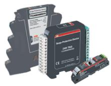
Combined Category D, C, B tested protector (to BS EN 61643) specifically designed for telecommunications applications in accordance with Telcordia and ANSI standards (see Application Note OVR AN005). For use at boundaries up to LPZ 0 to protect against flashover (typically the service entrance location) through to LPZ 3. Available as standard OVR TN format, or compact OVR TNQ and Slim Line OVR SL TN versions for installations where a high number of lines require protection.
