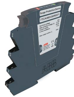
**Combined Category D, C, B tested protector (to BS EN 61643) suitable for twisted pair 4-20 mA loop systems with innovative LED protector status indication. For use at boundaries up to LPZ 0 to protect against flashover (typically the service entrance location) through to LPZ 3 to protect sensitive electronic equipment (e.g. transmitters, monitors, controllers).**
