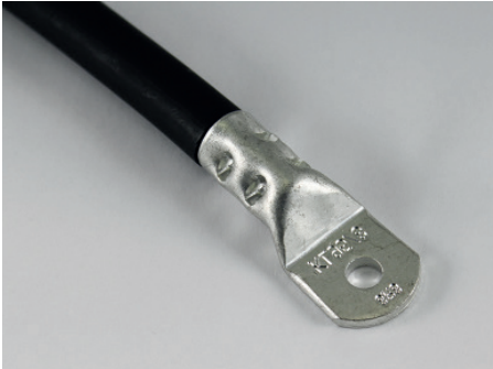
Fig.11: indent crimping; practical example
