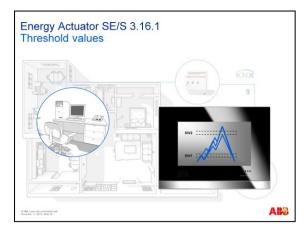
There are 2 threshold values available for each channel, and each threshold value has an upper and a lower limit. This enables a hysteresis function.
