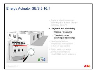
Active power, current and voltage, as well as other electrical variables (apparent power, reactive power, crest factor, power factor and frequency) can be measured for every channel.
