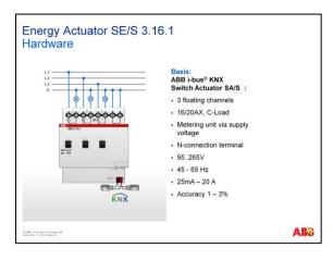
The Energy Actuator hardware is based on the tried and tested ABB switch actuators with the powerful C-load relay, there are 3 channels with 16 or 20 A and AX switching characteristics.
