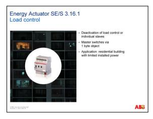
Whenever necessary, individual slave-channels can be removed via telegram from the load control and the entire control system can also be deactivated.
