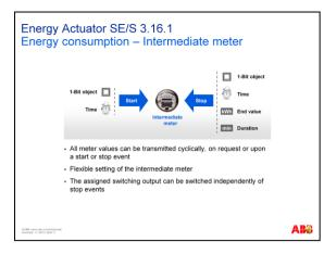
As we mentioned before, the meter values can be transmitted cyclically or on request. The Energy Actuator also allows the meter for example to start at a given time and after a certain operating time to stop automatically. A 1-Bit telegram or the time is available as a start and stop event.
