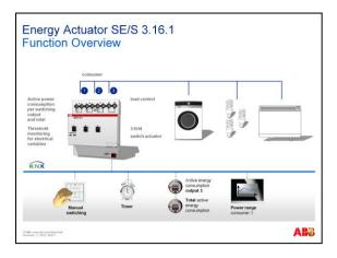
Following the switch actuator with current detection, ABB's Energy Actuator SE/S 3.16.1 represents the next level of intelligent actuators for ABB i-Bus KNX.
