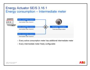
Besides the main meter every active consumption meter has an intermediate meter, to record for example daily consumption and the subsequent reset of the meter.
