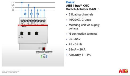
The Energy Actuator hardware is based on the tried and tested ABB switch actuators with the powerful C-load relay, there are 3 channels with 16 or 20 A and AX switching characteristics.
