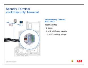
The 2-fold Security Terminal MT/U 2.12.2 differs from the previous components for distribution board mounting in that it is intended for decentralized installation e.g. in a wallbox. It has two inputs for zones as well as two 12 V outputs with a max. short circuit current of 0.6 A.
