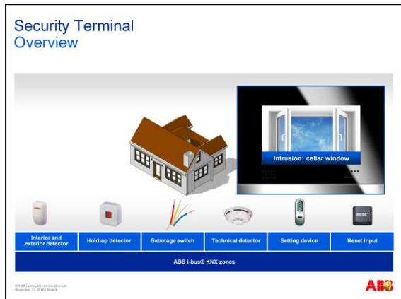
The types of zone can be adjusted as desired :
