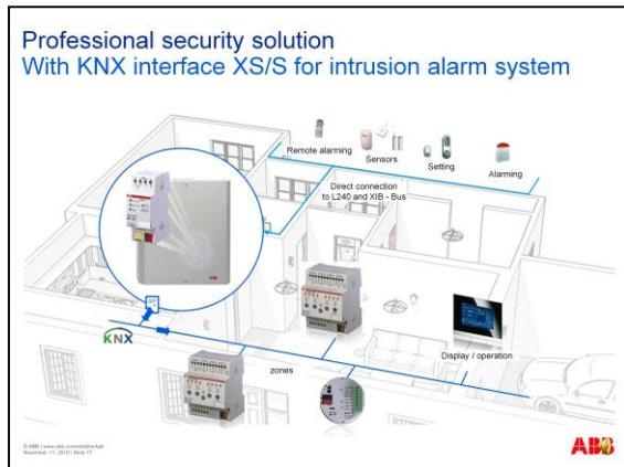
ABB's intrusion alarm panel L240 with KNX interface is another level in the integration of KNX and security technology. The L240 is an independent system with XIB security bus, to which all the required components can be connected.
