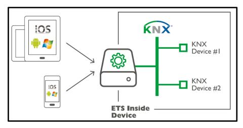
Basic principle of a decoupled user interface: Intelligent and simple parameterization via tablet or smartphone.
