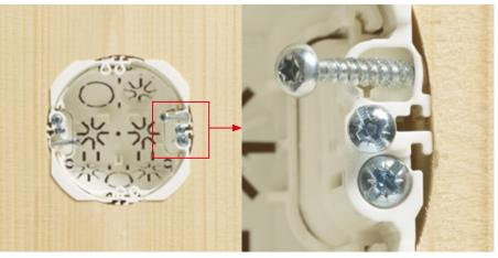
The box can be mounted on, for example, a timber wall or wooden frame with inclined screws (the maximum size of fastening screw head  $\emptyset$  6 mm).
