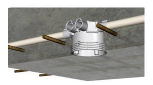
The overall height of the box is 73 mm which gives plenty of connecting space. The height from the conduit to the edge of the box is 47 mm. It is sufficient for the installation of piping above the reinforcements, without difficult and timeconsuming extra work.
