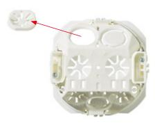
The strain relief can be modified for a flexible installation conduit by cutting it along the bottom of the box. It is easy and safe to cut using the bottom of the box. This way, the diameter of the hole is precisely 20 mm, as required for a flexible installation conduit.
