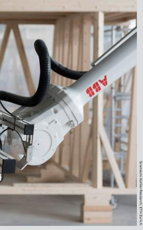
Wooden building modules are pre-fabricated in ETH's Robotic Fabrication Laboratory by two ABB robots equipped with PMA®'s cable protection products.
