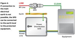
The ESP SPD should therefore be bonded to the main electrical earth or earth star point. The ESP SPD must be connected to earth via the bulkhead or right-angle brackets.
