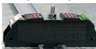
Figure 4: Installation on 'top hat' DIN rail.
