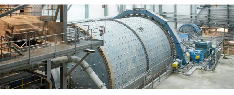
1,000 or 1,200 rpm. An asynchronous wound rotor induction motor with secondary starter is normally used to meet the high starting torque requirements. ABB has a complete range of gearbox and slip-ring motors, and can offer an optimized motor and gearbox solution for any type of mill application.
