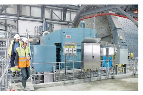
ABB's motors for mill applications are built for high levels of performance, quality and reliability in harsh conditions. They meet high demands for availability and help mining companies to operate mills continuously 24/7.
