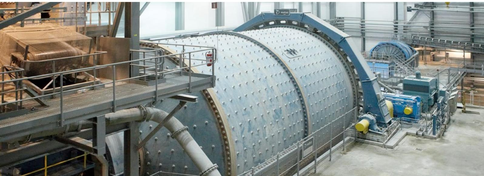
1,000 or 1,200 rpm. An asynchronous wound rotor induction motor with secondary starter is normally used to meet the high starting torque requirements. ABB has a complete range of gearbox and slip-ring motors, and can offer an optimized motor and gearbox solution for any type of mill application.
