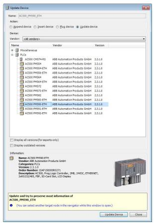
All sub nodes below the selected AC500 PM are automatically updated to the latest version 2.3.X in the device repository. The device update result is shown in the Message Window.
