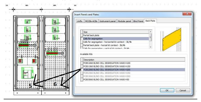
The user can evaluate the effective necessity to use the side rear segregations PLVS..., always inserted for this model with quantity 1, coherently with the horizontal kits segregations: if they are considered unnecessary ("product side" section) they must be manually removed from the items list.
