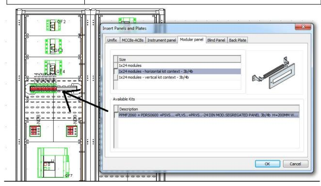
For the same reasons also the position below the DIN rail has to be occuped by a blind cell or a plate contextualized for this type of positioning:
