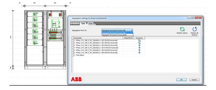
Clicking on OK button on the mask, the segregation process is automatically completed and the following picture shows the result (in case of use of segregation form 2 a - 3 a, the segregation direction has no meaning, so it is not necessary to indicate the direction in the segregation settings).
