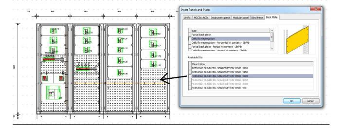
The blind cell placed in the third column at the height of the horizontal busbars must be of the simple type like shown in the image above. All the plates and cells result of the same height and coaxial.
