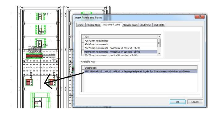
The same type of segregated cell or plate has to be defined for other zones with a vertical busbars passage. The segregation model also defines the necessary rear segregation for the cell.
