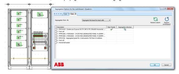
Abreast all the horizontally mounted devices, is admittable, both for 3b and in 4b forms, to choose for double indicator upward or downward.
