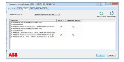
Concerning incomers (main breakers) usually (both for 3b form and 4b form) is required the spread of their own segregation orientation both upward and downward.
