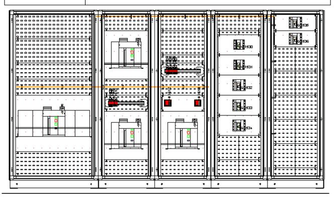
In the first three columns the segregation form 4b requires the use of segregated cells/plates with rear segregation over the entire width of the column (item PRVS...) and also 2 side rear segregations (item PLVS) related to the enclosure context: the software automatically introduce appropriate segregation kits.
