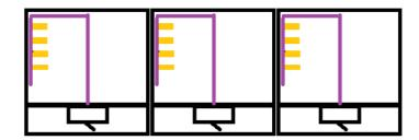
• In this further case the side segregations PLVS... aren't necessary for any columns. The busbars systems feed two adjacent columns and the dividers guarantee the rear side segregation (item PSVS...):
