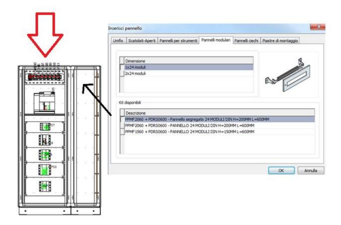
The software guarantees the possibility to introduce a specific segregation for blind, modular and instruments panels placed in the critical area between the incomer and its supply (clearly set in the upper side, as the red indicator shown).
