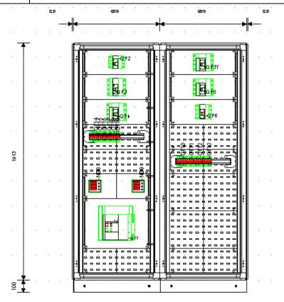
Empty spaces has been filled with segregate horizontal context back cells; furthermore, as a consequence, DIN panels and instruments panels introduced in the board front with simple segregation version, has been modified.
