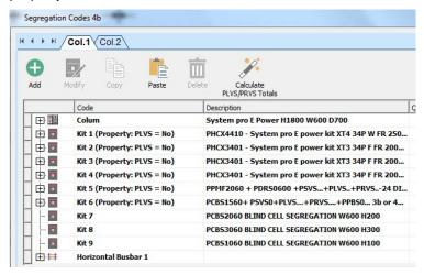
The value YES for property PLVS, stands for the presence on the kit of the segregation device shown in the picture below (seen from above):
