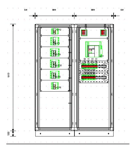
Automatically the software provides to combine kits and devices, verifying the compatibility between the type of the terminals and the required segregation form.
