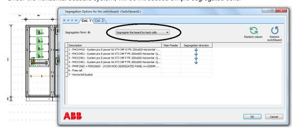
On the second column instead, is installed a main circuit breaker vertically mounted: the automatic functionality will complete the segregation with vertical context cells (both upward and downward, as declared by the indicators) till the intersection with horizontal busbar system.
