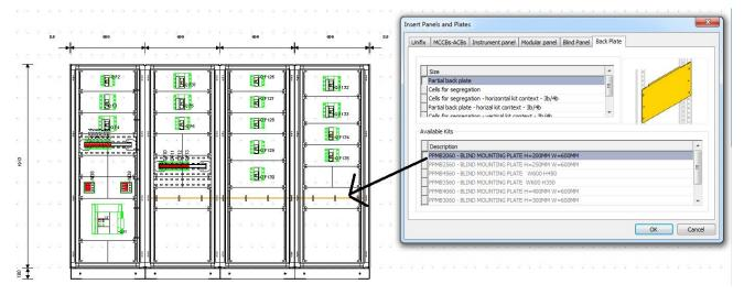
Above the picture represents the result in case of using plates, instead of cells, to segregate.
