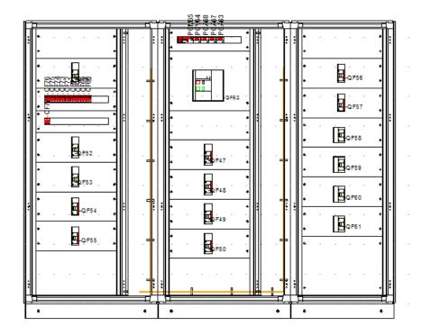
All the mounting kits related to moulded case or air circuit breakers placed in the enclosure are automatically completed with the necessary segregation items (rubber covers, items PPRS..., for molded case circuit breakers, specific segregations for Emax 2 with rear terminals).
