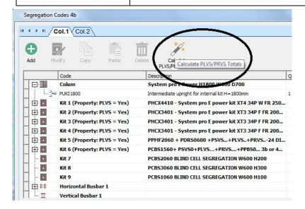
PRVS/PLVS total height codes, are introduced beneath column node, meanwhile corresponding accessories in single kits are deleted.
