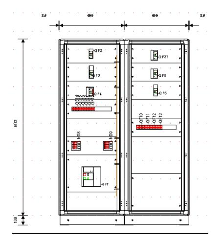
All the mounting kits related to molded case or air circuit breakers placed in the enclosure are automatically completed with the necessary segregation items (items form 2a - 3a + further segregation elements form 3b – 4b).
