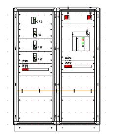
4b form segregation requires an appropriate completion of the switchboard in plates layer.
