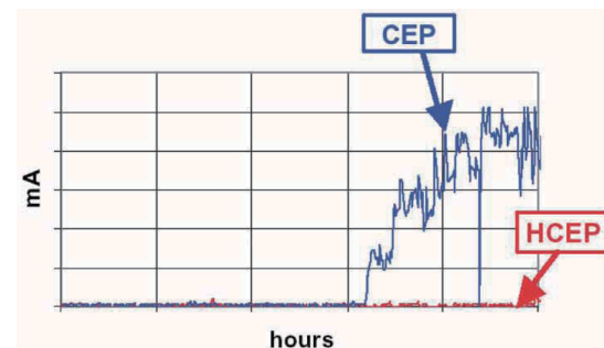
Comparison of CEP and HCEP after 1000 hours salt-fog test
