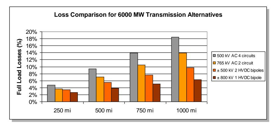
Note: AC and DC line conductors chosen for comparable current densities, higher no. conductor bundles for higher voltage.
