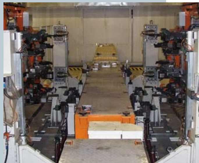
FlexFramer technology from ABB allows for flexible laser production at SVW.
