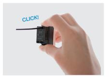
Release the pusher and check the fastening.
