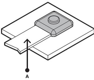
The diagram shows a cross-section of a flat tape conductor being inserted into a mould. An arrow labeled 'A' indicates the direction of insertion.
