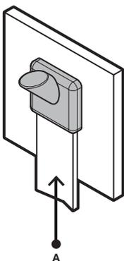
The diagram shows a cross-section of a flat tape conductor being inserted into a mould. An arrow labeled 'A' indicates the direction of insertion.
