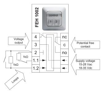
Control units FEH1001 and FEH1002 include a separate cancel button and a signal light for each loop. Control unit FEH1101 has a switch instead of the button and therefore the loop can be disconnected. In an alarm situation the signal light flashes and when reset or disconnected it will light steadily. The signal light can be tested using the button.
