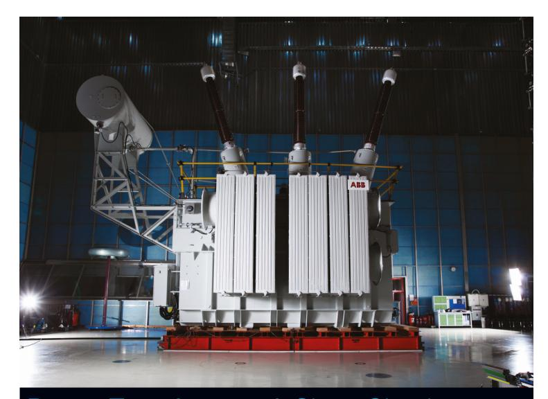
Power Transformers & Short Circuits Evaluation of the short-circuit performance of power transformers
