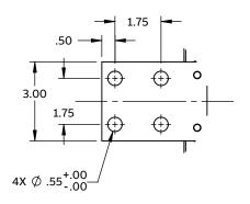
DETAIL E SCALE 1 : 4 GROUND AND NEUTRAL BUS DETAILS
