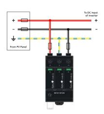
IMPORTANT: In order to protect sensitive electronic equipment, particularly from electrical switching transients, plus ensure the continual operation of systems, full mode SPDs, with both common and differential mode protection, are required. ESP M1 Series or ESP D1 Series SPDs should be installed at AC sub-distribution boards feeding sensitive equipment. For further information, please refer to the Furse Guide to BS EN 62305 Protection against lightning.
