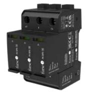
Type 2 tested surge protective device SPD (to BS EN 61643-31) for DC applications such as Photovoltaic PV solar panel systems. Typically for use at the DC side of the DC-AC inverter located within lightning protection zone 1 LPZ 1 to protect the PV system from surge damage due to lightning and electrical switching events.
