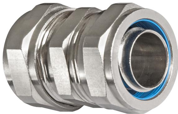
Type U/M liquid tight, nickel plated brass coupler with co-polyester seals. Suitable for coupling separate lengths of liquid tight conduit together.
