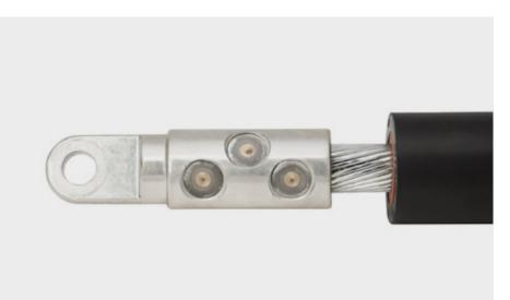
The Elastimold™ advanced shear bolt connection system provides a highly reliable solution for 600 A and 900 A elbow connectors that helps reduce the likelihood of installation error with the shear bolt connector's range-taking capability.
