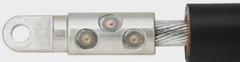
The Elastimold™ advanced shear bolt connection system provides a highly reliable solution for 600 A and 900 A elbow connectors that helps reduce the likelihood of installation error with the shear bolt connector’s range-taking capability.
