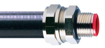
Stainless steel 316 straight fitting, external male thread. For insertion into threaded entries or knockouts using a locknut to secure.
