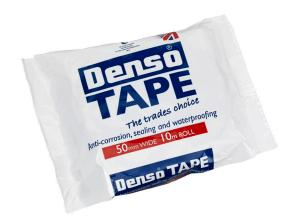
Denso Tape is a grease saturated, non-hardening and non-cracking fabric tape that is used, amongst other things, for the protection of buried conductor joints in earth electrode systems.
