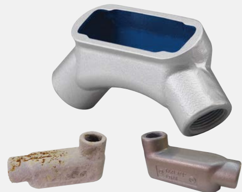
After a 500-hour 5% salt fog test, the standard galvanized iron conduit body has severe salt adhesion and significant rusting.
