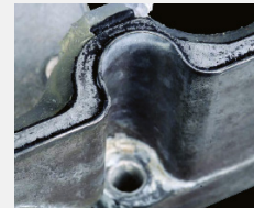
The edge of a CorroStall® aluminum alloy conduit box after the same salt spray test.
