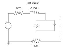
The applied voltage was selected at 27.5kV, much in excess of normal line-to-ground voltage, to increase the failure rate. This allowed evaluation of test and design parameters with a limited number of samples.
