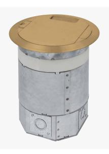
Recessed service, 5-gang pokethrough designed to fit in 8" holes in the second floor and above in commercial buildings. Given the limitations on the number of holes that can be drilled in a floor, it is important to maximize the capacity of each location. The RPT8 Series offers a configurable solution that provides high capacity for both power wiring and communications cabling—in a single-core drill location.
