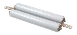
Commonly used on 34.5 kV and lower systems to enhance protection, external current-limiting backup fuses coordinate with series expulsion fuse to offer very high interrupting capability and reduce energy let-through during a fault. The proven benefits of the two-fuse approach widely used on distribution systems is now available for application up to 138 kV that traditionally only protected by a standard expulsion fuse.
